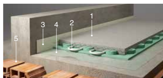
1 - screed with electro-welded mesh 2 - layer of thermo-acoustic insulation 3 - perimeter joint 4 - polythene sheet 5 - weight-bearing structure (floor)
