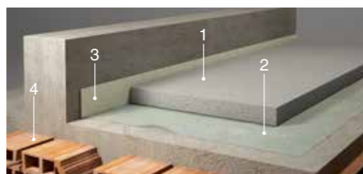
1 - screed 2 - polythene sheet; 3 - perimeter joint 4 - weight-bearing structure (floor)
