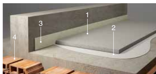
1 - screed 2 - adhesive cement slurry 3 - perimeter joint 4 - weight-bearing structure (floor)
