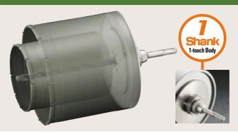
Adopts unique double blade features, with the inner-blade preceding the outer-blade, therefore, boring through material such as; metallic siding, stainless steel/wood siding as well as compound materials (metallic plate + insulating material + plywood) at one go is possible. Swarf is efficiently discharged in boring wooden materials. It is also
