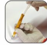
Put into handle kerosene or other suitable lubricants and screw tight cover
