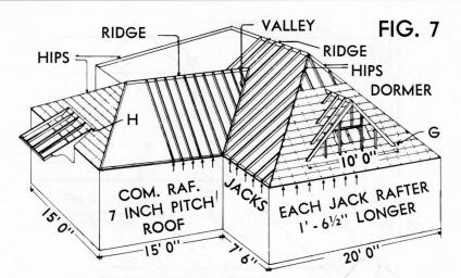
ALL CUTS ON THIS ROOF MADE BY USING THE NUMBER 7 (INCH RISE)
