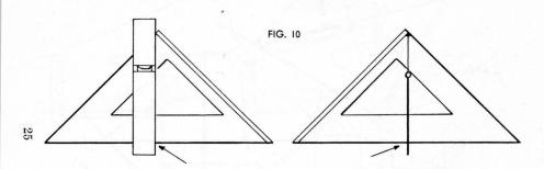
PLACE A 7" (OR LONGER) LEVEL ON FACE OF SQUARE WITH TOP EDGE OF LEVEL ALWAYS RESTING AGAINST """ BAR AT PIVOT POINT ON SQUARE. SUBBLE SHOULD ALWAYS INDICATE THAT THE LEVEL IS BEING HELD PLUMB. PIVOT SQUARE FROM EDGE OF LEVEL. USING THE LEVEL AS A PLUMB LINE WILL GIVE FASTER READINGS BECAUSE YOU DON'T HAVE TO WAIT FOR THE SYNINGING MOTION OF THE STRING (AS USED IN THE NEXT METHOD) TO STOP. ARROWS INDICATE POINT AT WHICH DEGREE IS SHOWN.
