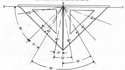
LINE X-Y REPRESENTS EDGE OF MATERIAL, POINT B IS PIVOT POINT OF SQUARE. HERE SQUARE IS NOT PIVOTED, POINTS ARE MARKED ON MATERIAL AT POINT B, AND AT DESIRED ANGLE. LINE DRAWN THRU THE TWO POINTS GIVES THE ANGLE WANTED.
